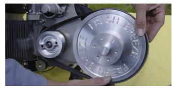
If the belt makes squeaking noises in spite of the proper tension, then spray twice onto the lower pulley. If the belt is slipping in spite of proper tension, then it needs to be replaced.
