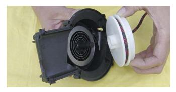
The starter-rope can be pulled out of the disc.
