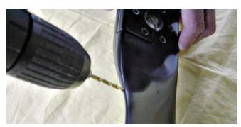
Then fill only as much resign into this hole until the propeller doeas not want to turn to one side only.
