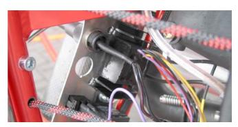
Via this plug a voltage can be transmitted. The dynamo has a limit of max.  $24\ VA$ .
