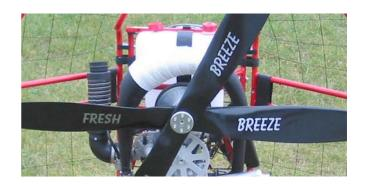
The complete exhaust is suspended flexibly as to prevent vibrational eruptions.
