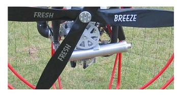
To keep the exhaust flexibly mobile we chose different types of fixtures. One is a rubber connection on the gear-plate and two a stress-bearing spring-gasket at the entry and the exit.
