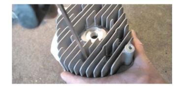
To reopening the hole use a 3,5mm drill. Bore from top and from inside the cylinderwall with an angle from  $45^{\circ}$ .
