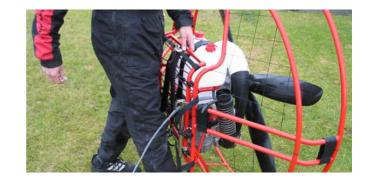
The cage should fixed against the frame with the velcro.
