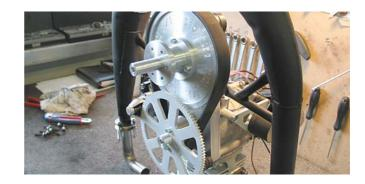
During maintenance check the belt before each flight. The belt should not be able to be turn over 45° degrees. After the first flight it is essential to pay special attention to the belt.
