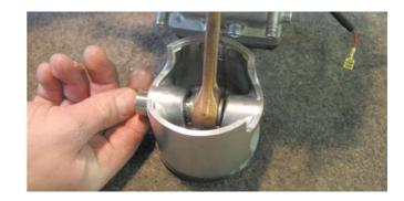
The pistonring can removed by hand.
