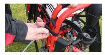
After assembling all velcro's should tighten again.
