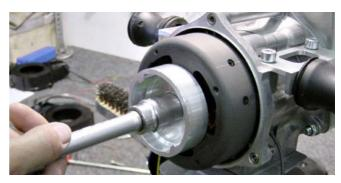
To fine-tune the ignition timingpoint one has to loosen the two security screws of the stator. Turn the stator to the left maximally to the furthest point, now turn ca 2 mm to the right again. Retighten the security screws. The ignition timingpoint has now its correct adjustment. When reassembling take special care of the correct distance of the contact-test that the distance of 0,25 mm is observed and if nessecary readjust.
