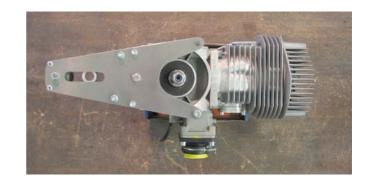
In flight the motor will become very hot. The most stressed airea are the piston and the rings.Remove the exhaust and have a look to appearenced piston with it's rings. Test it with screwdriver.The rings should be loose inside the slot.
