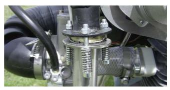
After 10 hrs the sealing-rings and their fasten screws needs to be checked. The screw you have to changes each  $25\ hrs.$
