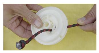
To give the starter-rope advanced tension one,place the rolled up into the slot and rotate three times.
