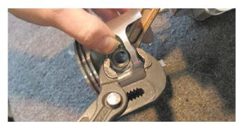
To the piston belongs two different rings. The upper ring is marked with a "O". This is faced to the top.
