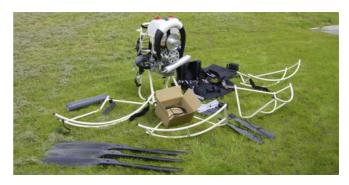
Bring the four cageparts together and fix with velcostraps.
