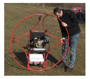
The starter rope needs to be fitted to the shackle in the upper cage
