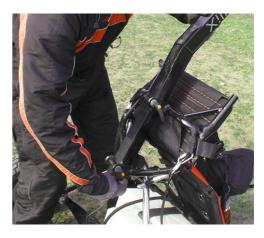
The rear wheels are easily removable for transport. The inserted spindle is secured by clip pin.
