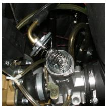
The needle 6L1 is mounted in the second position
