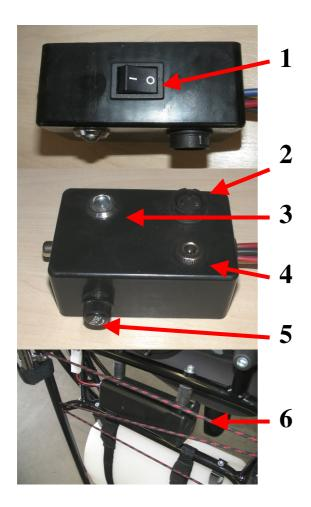
The motor can be equipped with an alternator. This includes an E-box and a battery. The batterie is recharged in flight. The E-box includes the following:
