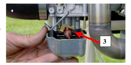
With an 8 mm wrench the mainjet (2) can changed. Number 3 is the fuel mixture jet size 60
