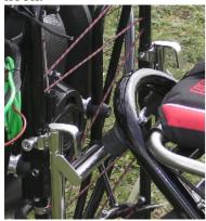
The multi-tubes must fit properly in the white clips. Be aware that the centering pins fit into the holes of the multi-tubes
